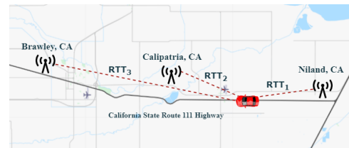
Fig. 3: Part of a real-world 5G commercial topology located near State Route 111 highway, California U.S.
